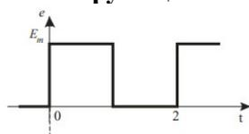
$$e(\omega t) \approx \frac{E_m}{2} + \frac{2 \cdot E_m}{\pi} \cdot \left( \sin \omega t + \frac{1}{3} \sin 3 \omega t + \frac{1}{5} \sin 5 \omega t + \dots \right)$$
