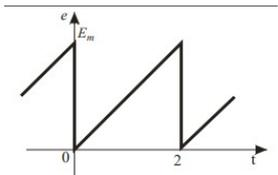
$$e(\omega t) \approx \frac{E_m}{2} - \frac{E_m}{\pi} \cdot \left( \sin \omega t + \frac{1}{2} \sin 2 \omega t + \frac{1}{3} \sin 3 \omega t + \dots \right)$$
