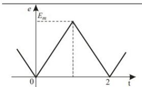
$$e(\omega t) \approx \frac{E_m}{2} - \frac{4 \cdot E_m}{\pi^2} \cdot \left( \cos \omega t + \frac{1}{9} \cos 3 \omega t + \frac{1}{25} \cos 5 \omega t + \dots \right)$$
