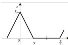
$$e(t) \approx \frac{E_m}{2} + \frac{4 \cdot E_m}{\pi^2} \cdot \left( \cos \omega t + \frac{1}{2} \cos 2 \omega t + \frac{1}{9} \cos 3 \omega t + \frac{1}{25} \cos 5 \omega t + \dots \right)$$
