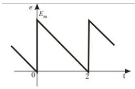
$$e(\omega t) \approx \frac{E_m}{2} + \frac{E_m}{\pi} \cdot \left( \sin \omega t + \frac{1}{2} \sin 2 \omega t + \frac{1}{3} \sin 3 \omega t + \dots \right)$$
